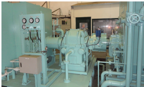
High Speed Gearbox for Steam Turbine Generator Drive, up to 80MW.
