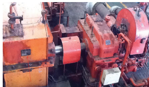
High Speed and Secondary Helical Gears for Pressure Feed Drive.
