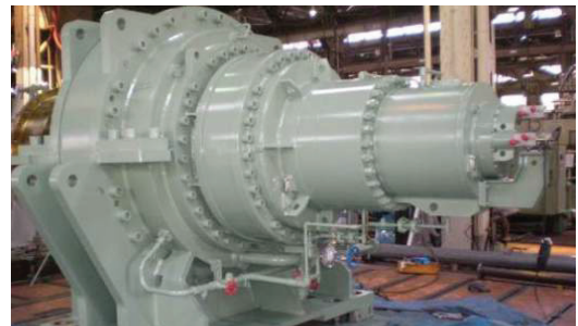
Large Planetary Gearbox for Mill Drive and Pressure Feeder Drive.
