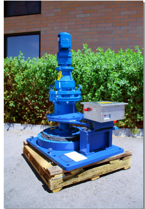
Figure 6: Vertical Cyclo® Speed Reducer is mounted to a base, waiting to be installed atop a clarifier
