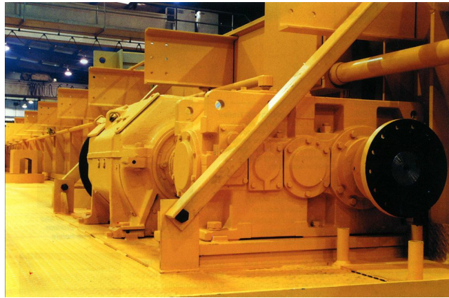
Figure 4. 100' span bridge crane with Sumitomo Paramax® reducers 3
