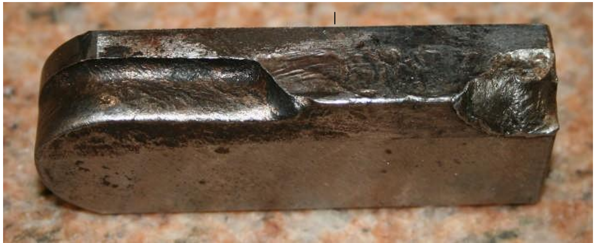
Damaged Paramax Speed Reducer Key
