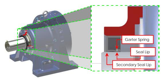
Since these seal lip(s) are riding against a rotating shaft (or collar), friction at this interface is developed, hence, an energy loss (albeit small) is realized. The amount of this energy loss due to friction is dependent upon many factors that include shaft speed, shaft diameter, and the surface finish/roughness against which
