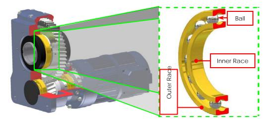
As noted, a bearing is a <u>low-friction</u> device, it is not friction-free. As one race rotates about the other race, the balls (or rollers) likewise rotate/slide within the race. The rotating/sliding action of the balls (or rollers) creates friction between these bearing components thereby creating an additional avenue for energy loss.
