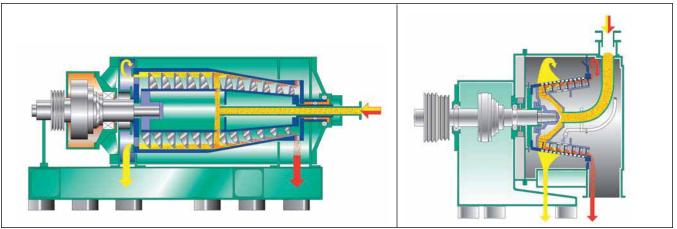
Figure 1-Decanter (closed-bowl) centrifuge.
