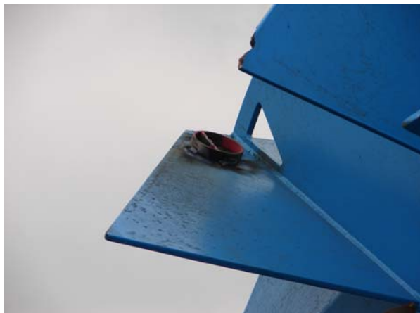
Figure 9. Added Weight to Re-Balanced Aerator 1
