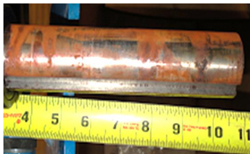
Figure 1: Fretting condition example. Staining is an evidence of fretting occurrence.
