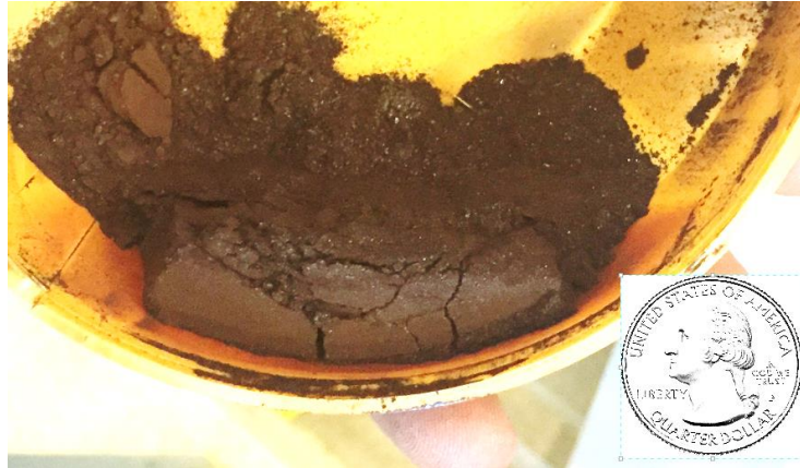
Figure 3: Fine oxide powder as a result of fretting
