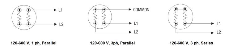
Figure 2:Wiring Diagrams
